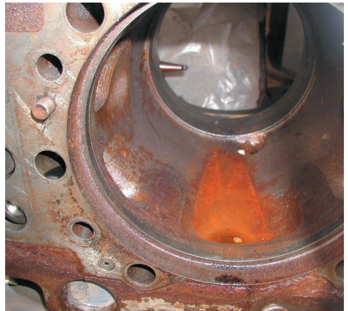
Aangetaste cilinderwand motorblok. © Materials Consult.
